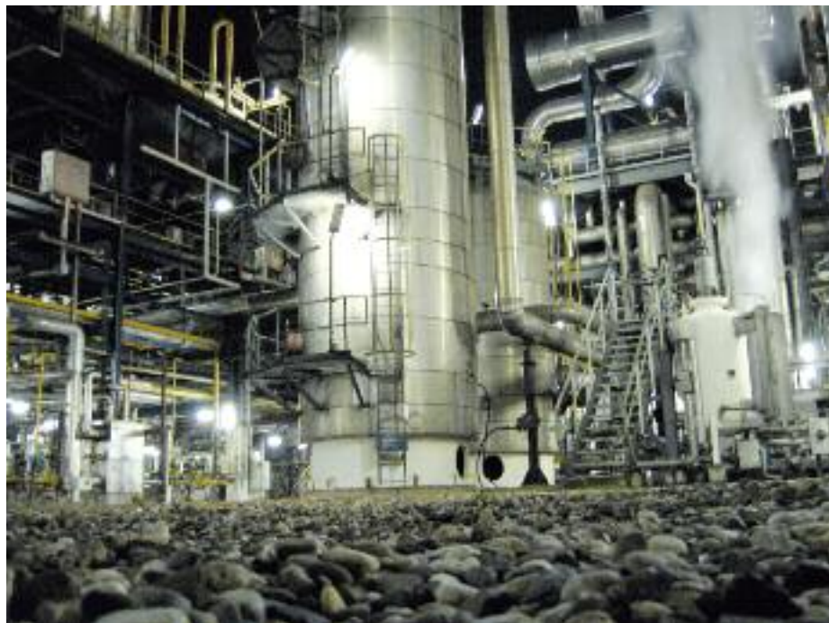
BioMCN produces bio-methanol from glycerine, a by-product from producing bio-diesel, on a large industrial scale
