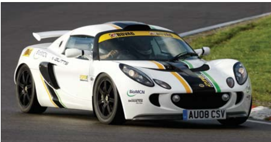
The Lotus Exige 270E Tri-fuel is capable of running on any mixture of gasoline, ethanol and (bio)methanol
